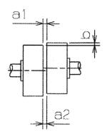
Figure 3. Mounting of half-coupling or pulley
