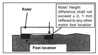
Before mounting the motor, the foundation surface for the shims or for the feet must be clean from thick paint, paint drops and dirt. Then it should be checked in order to discover any height differences between the individual foot locations. Also, the smoothness within each footprint area has to be checked. The requirements are noted in the figure below.
