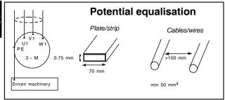
To comply with EMC-requirements, use only cables and connectors approved for this purpose. (See instruction for frequency converters.)
