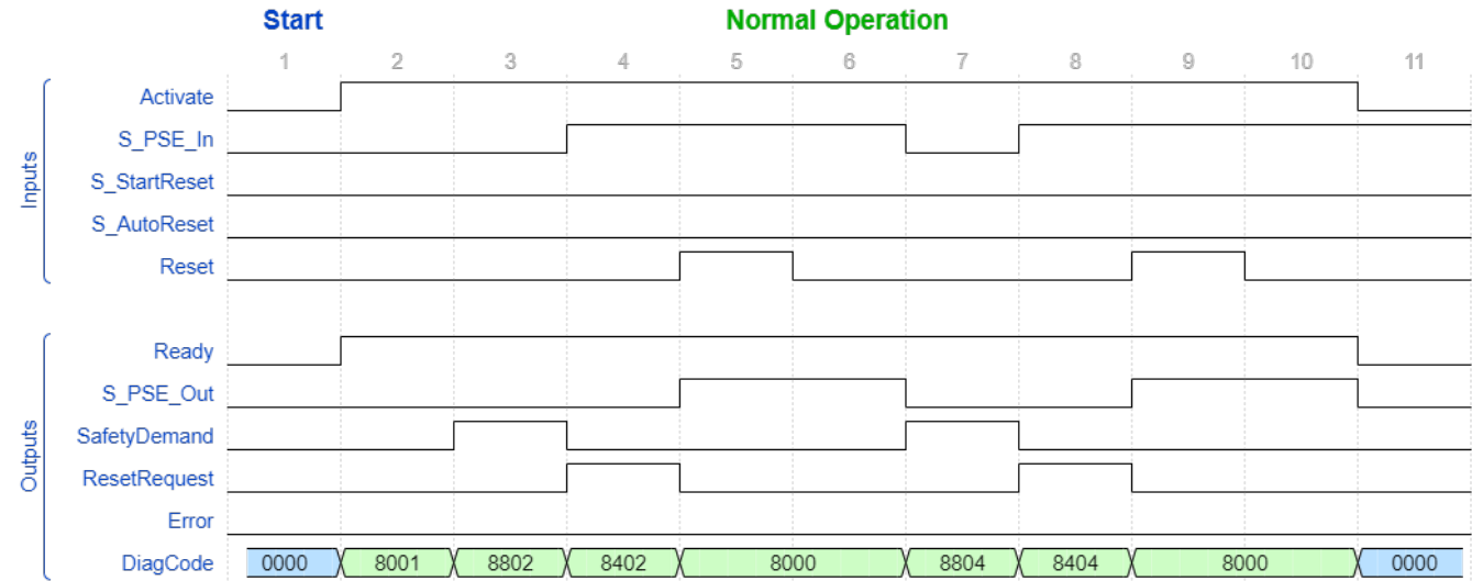
Fig. 105: Typical timing diagram for SF_PSE: S_StartReset = FALSE, S_AutoReset = FALSE
