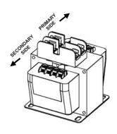
ORIENT THE FUSE-HOLDER SO THAT IT WILL BE LOCATED ON THE SECONDARY SIDE OF THE TRANSFORMER. (SEE STEP 2 FOR ACTUAL ASSEMBLY)
