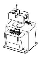
USE THE #6 SCREW PROVIDED TO MOUNT THE FUSE-HOLDER DIRECTLY ON TOP OF THE TRANSFORMER. THE SCREW WILL GO THRU THE FUSE-HOLDER, THRU THE MOUNTING BRACKET AND INTO THE TRANSFORMER MOUNTING TAB.
