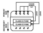
CONNECT A LEAD PROVIDED TO ONE SIDE OF EACH OF THE CLASS CC FUSE-HOLDERS AND TO THE APPROPRIATE PRIMARY TERMINALS OF THE TRANSFORMER.
