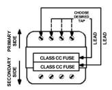
1) CONNECT A LEAD PROVIDED TO ONE SIDE OF EACH OF THE CLASS CC FUSE-HOLDERS AND TO THE APPROPRIATE PRIMARY TERMINALS OF THE TRANSFORMER.
