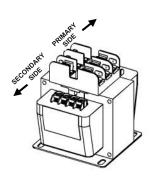
ORIENT THE FUSE-HOLDER SO THAT IT WILL BE LOCATED ON THE SECONDARY SIDE OF THE TRANSFORMER. (SEE STEP 2 FOR ACTUAL ASSEMBLY)
