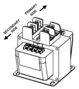
ORIENT THE FUSE-HOLDER SO THAT IT WILL BE LOCATED ON THE SECONDARY SIDE OF THE TRANSFORMER. (SEE STEP 2 FOR ACTUAL ASSEMBLY)
