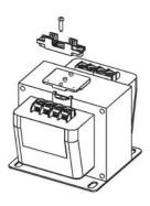
USE THE #6 SCREW PROVIDED TO MOUNT THE FUSE-HOLDER DIRECTLY ON TOP OF THE TRANSFORMER. THE SCREW WILL GO THRU THE FUSE-HOLDER, THRU THE MOUNTING BRACKET AND INTO THE TRANSFORMER MOUNTING TAB.
