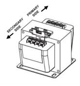
ORIENT THE FUSE-HOLDER SO THAT IT WILL BE LOCATED ON THE SECONDARY SIDE OF THE TRANSFORMER. (SEE STEP 2 FOR ACTUAL ASSEMBLY)
