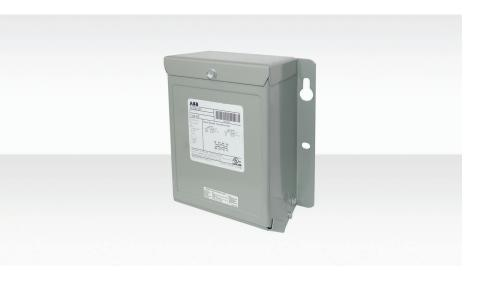
Buck-boost transformers are small, single-phase, dry type distribution transformers designed and shipped as insulating/isolating transformers. They have a dual voltage primary and a dual voltage secondary. These transformers can be connected for a wide range of voltage combinations.
