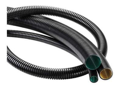
The new PMA multilayer technology allows combinations of materials for optimal product characteristics in rail applications. An innovative multilayer manufacturing technology creates a corrugated conduit with two layers of material. This multilayer solution provides additional protection and safety thanks to the combination of two specially modified polyamides with different material characteristics. The new material combinations significantly improve the overall performance of the conduits.
