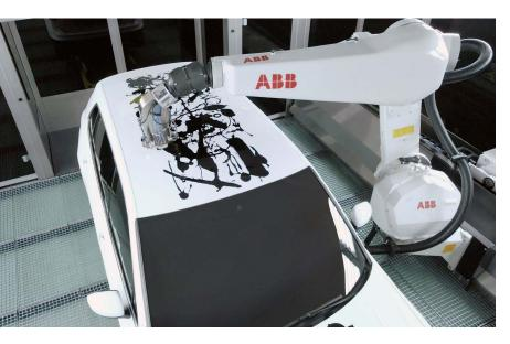
ABB's PixelPaint non-overspray technology helps auto makers respond to the demands of car buyers. When creating popular twotone or customized paint jobs, it eliminates the need for time-consuming masking and demasking. This significantly reduces time and cost, while also improving productivity and expanding the possibilities of customization.
