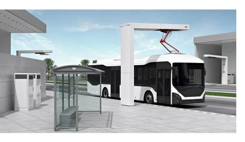
ABB's HVC-PD opportunity charging system offers high-power charging via an automated rooftop connection. With typical charge times of 3 to 6 minutes the system can be easily integrated in existing operations by installing chargers at endpoints, terminals and intermediate stops.
