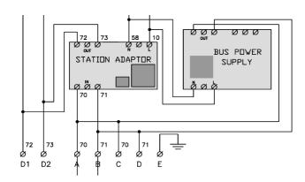
The MXKP station adapter kit is required to integrate the EMEX Power static inverter with the EMEX Test system. It is ordered separately, the MXKP station adaptor kit is fitted in the inverter cabinet.
