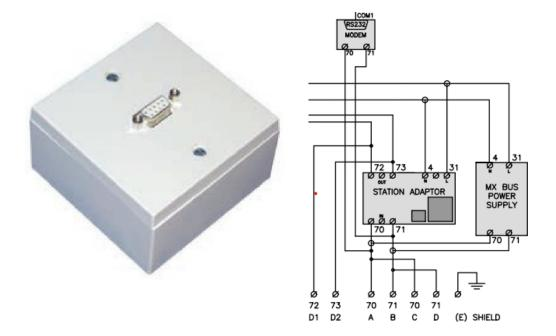
The EMEX Test Modem provides an input point for allowing roving access to the system using a laptop or PC.
