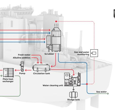
In a **hybrid scrubber arrangement**, both open-loop and closed-loop modes are readily available. Open-loop operation reduces costs whenever possible, but a switch to closed-loop operation can be made whenever local water discharge regulations demand it.
