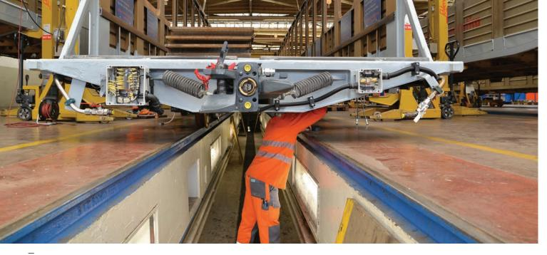
01 Major requirements for flexibility, impact resistance and corrosion protection. Car transporter wagons are retrofitted with PMA cable protection solutions.
