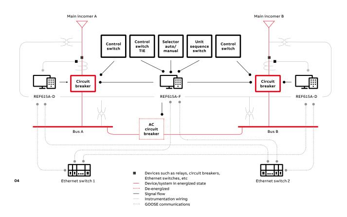
04 Typical single-line diagram of an M-T-M ATS configuration. concept that includes the entire protection, control and supervision system as well as cyber security – using just one protocol.
