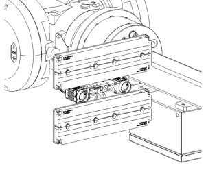
The Compliant Vision Guidance (CVG), with one or two cameras embarked on the robot tool, taking captures in a range of 30-40 Hz, compensates residual deviations over the pseudo static environment achieved by the UVT.
