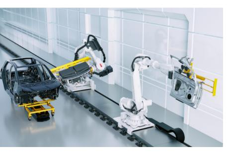
Dynamic Assembly Pack enables automating assembly processes in continuous movement, for any transport system despite irregularities and uneven floors that result in shaking and vibrations. And with maximum flexibility to cope with any variant.
