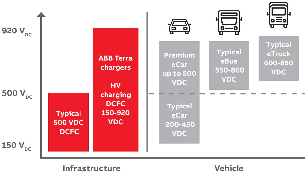
A high range of DC voltage capability is demanded to deliver efficient charging service to every EV and use case.
