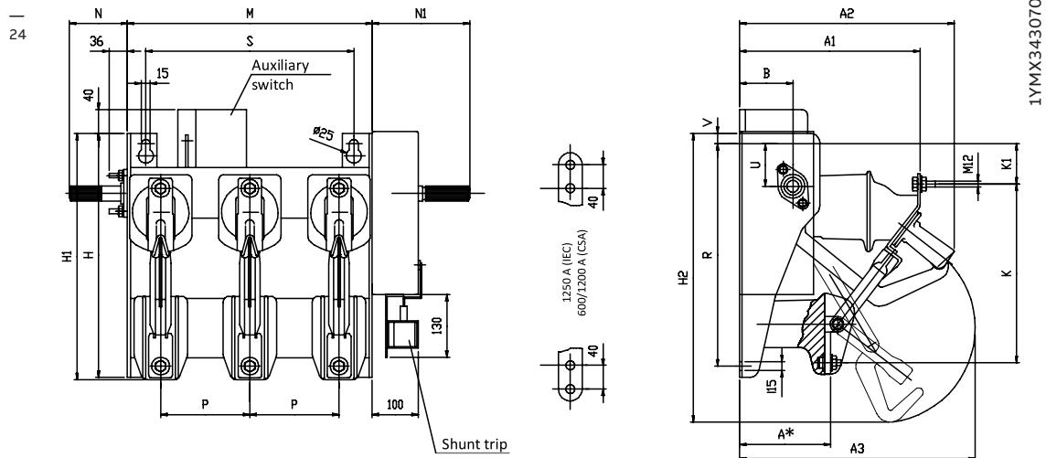
**Switch-disconnector type NAL-H (12, 17 and 24) IEC with mechanism**
