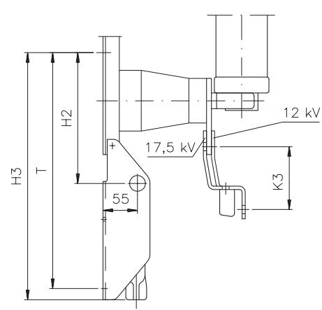
Earthing switch mounted on the fuse-base
