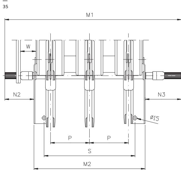
Earthing switch mounted on the switch-disconnector
