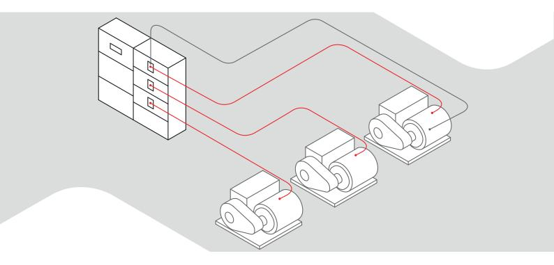
'Starting', 'Switching' and 'Protecting' are main three concerns when designing systems with three-phase asynchronous motor.
