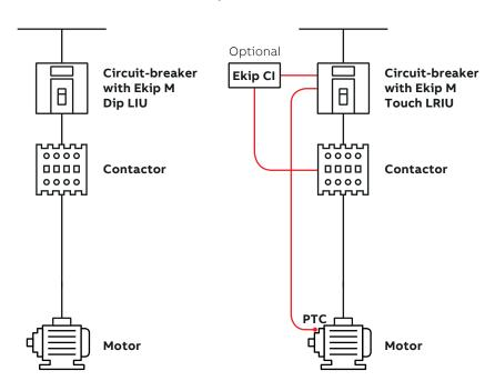
The following are few of the solutions that can be provided with circuit breaker for short-circuit protection, a thermal relay for overload protection and a contactor for motor switching.
