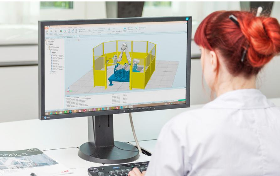
Computer-based programming is the best way to maximize return on investment for robotic systems, resulting in lower costs, faster time to market and superior end products. ABB RobotStudio® allows programming to be done on a computer without disturbing existing production.
