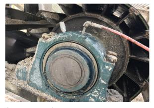
Smart sensors (shown here as the white cylinder on the bearing) allow equipment to be monitored in locations which may be difficult or dangerous to reach.
