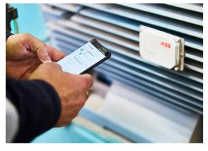
Smart sensors monitor key parameters to provide detailed insights into the performance and health of motors. As a result, maintenance can become predictive rather than reactive.
