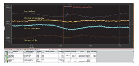
Domtar was able to maintain wet end ash stability during sheet breaks by utilizing headbox and silo ash percentage measurements.
