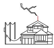
• Galvanic coupling occurs when lightning hit a lightning rod or the roof of a building.
