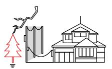
• Inductive coupling occurs in two main scenarios, when lightining hits a roof equipped with earthing system or when lightning takes place near some aerial electric lines causing an overvoltage that propagates in each near circuit.
