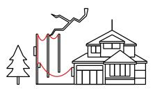
• Conductive coupling occurs when lightning hit an aerial electric line or a low voltage line.
