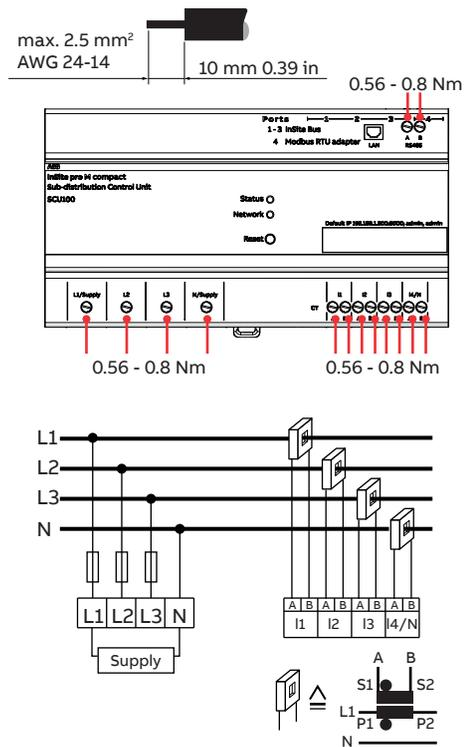
Install device single phase (L1-N) or three phase (L1, L2, L3, N)
