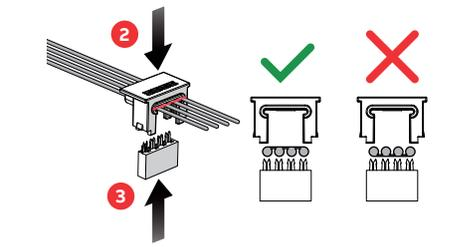
**Attention:** Pay attention to the correct orientation of the cable. Make sure that the cable is properly inserted into the connector housing.
