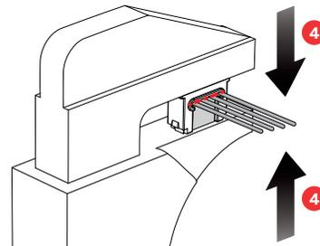
Plug connectors to Control Unit and sensors/I/O modules
