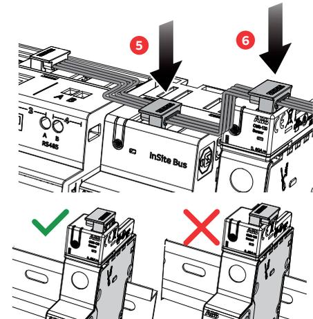
**Attention:** When plugging in the InSite flat cable on the modules, check the correct connection direction.
