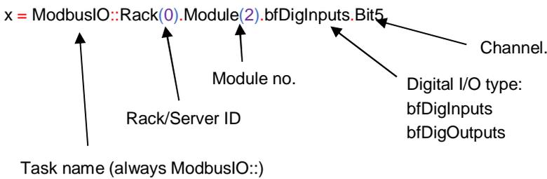
As another example, to turn on output C19 on this same module the Mint code would be of the form: ModbusIO::Rack(0).Module(2).bfDigOutputs.Bit19 = \_On
