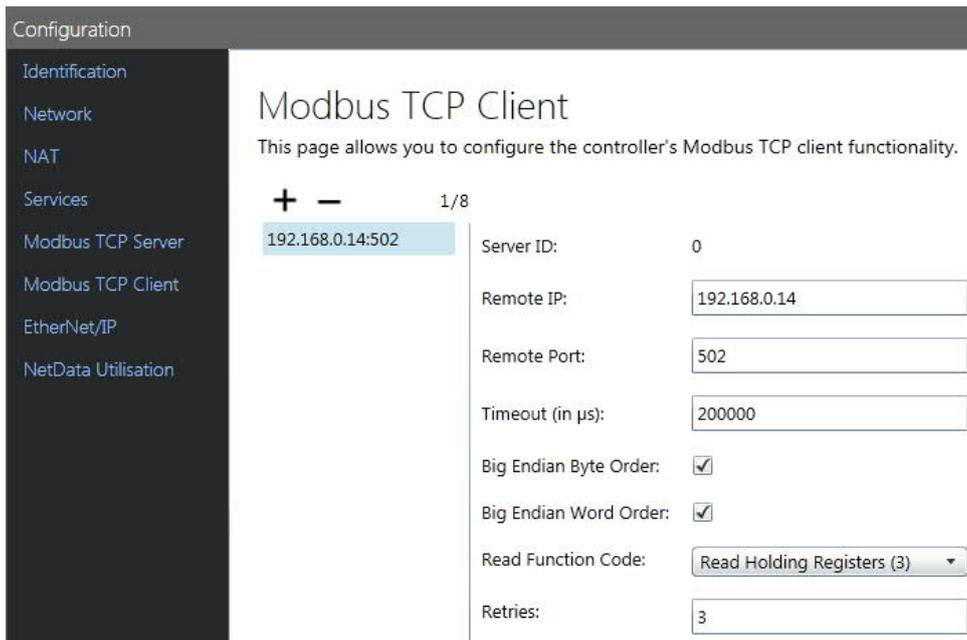
Click on the '+' button to add the second logical I/O rack to the configuration (this is I/O Rack 1 so the server ID for this rack must also be 1). This rack is headed by the CI522 module and the IP address for this module has been set (via its rotary switches) to 192.168.0.15 so this is the value we enter for the Remote IP address...
