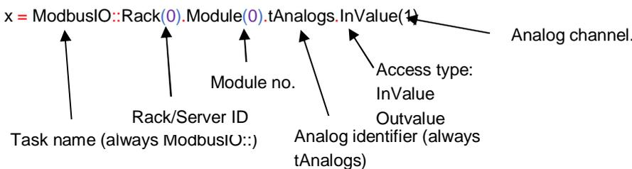
...and to write to analog output 0 on this rack/module (e.g. to set 52.3%) we would use code of the form...
