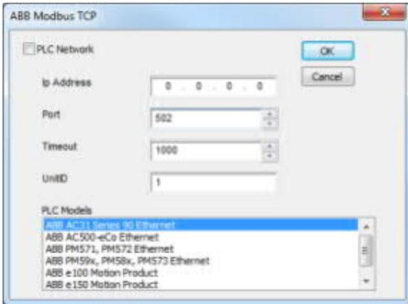
If the HMI is connected to a single Modbus TCP slave device (e.g. MicroFlex e190 or AC500 PLC) there is no need to select the 'PLC Network' check box. If there are multiple slave devices connected to the HMI then it is essential this box is selected (for the purposes of this application note we will select this option).
