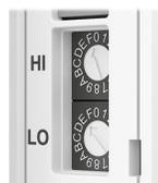
The rotary switches on the drive should be set to the required EPL node number. Any unique value from 1 to 239 (01 to EF hex) can be used.
