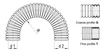
stat. R. = min. bending radius for static (fixed) installation
