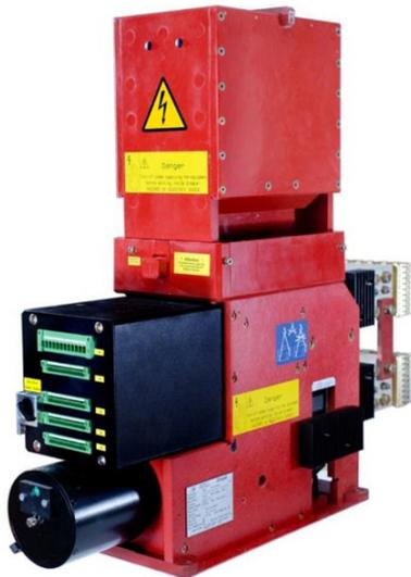
Gerapid is a single pole, high-speed, DC air circuit breaker designed for use in DC traction power substations. The combination of high interruption capacity and current limiting characteristics makes Gerapid a reliable protection solution for high-power DC power distribution systems.
