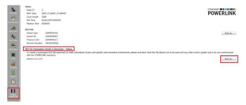
Now start Automation Studio (AS 4.3.6.57 or later). From the Tools menu select 'Import Fieldbus Device' and navigate to the XDD file saved previously. Once imported, the drive (MicroFlex e190 or MotiFlex e180) will appear in the 'Third Party Devices' section of the AS device catalog.
