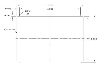
Figure 20: M2X–M6EX cut-out template
