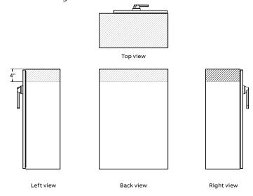
Figure 6 — Standard: top feed TG3 products (metallic enclosure, NEMA 4/12)
