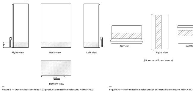
Figure 8 — Option: bottom-feed TG3 products (metallic enclosure, NEMA 4/12)
