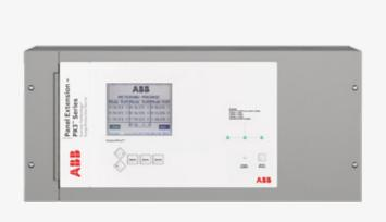
The PX3™ offers an externally mounted surge solution that can be physically attached to the top or bottom of any panelboard, providing a reduced profile surge solution. PX3™ suppression filter systems feature a powerful failure-free ISM™ (Integrated Suppression Module). The ISM™ contains individual thermally fused and protected MOVs, surge-rated copper busing, robust filtering and advanced remote communications capabilities.
