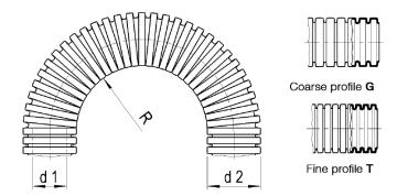
stat R. = Lowest recommended bending radius for static (fixed) installation
