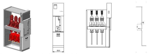
1 Panel type HBS, LSC2 - Circuit-breaker with switch-disconnector integrated - 500 mm
