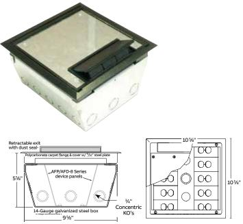
AFM-8 Shown with optional power panels (sold separately). Accepts 10 device panels. Each compartment can accept voltage dividers for any combination of power and data (included with device panels).
