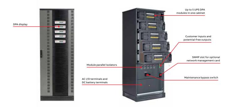
The Conceptpower DPA is a true double conversion modular UPS designed for medium-sized critical applications. The Conceptpower DPA's modular architecture provides very flexible power configuration based on 30/40/50 kVA modules that can be added as power requirements grow –
