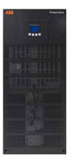
The PowerValue 11/31 T UPS delivers reliable power, low running costs, long battery life, easy maintenance and high levels of flexibility. Featuring double-conversion, voltage and frequency independent (VFI) topology, the PowerValue 11/31 T is available in both 10 and 20 kVA versions, with the option to configure up to four units in parallel to boost power capability or provide redundancy.
