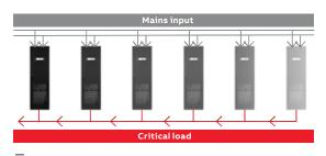
Up to 10 units can be configured in parallel to provide up to five megawatts of UPS power or redundant backup. This scalability means the UPS system capacity can be sized to match the load requirements, with the possibility to add incremental capacity later, when power needs change. The resulting savings in power usage over the service life of the UPS are substantial.
