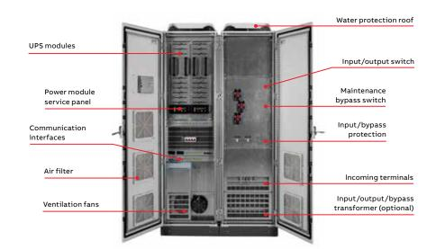
PowerLine DPA (3ph and 1ph) is an online double conversion UPS and makes the advantages of ABB's unique modular UPS architecture available for locations that are usually rough on electronic equipment. PowerLine DPA is based on ABB's Decentralized Parallel Architecture (DPA) that ensures the very best UPS design in terms of availability, serviceability, safety and ease of use.
