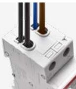
Supply operation is allowed in parallel with busbars and cables (either from top or bottom side) as terminals are composed of two different seats: a front seat for 25 mm2 cables and a back seat for 10 mm² busbars.
