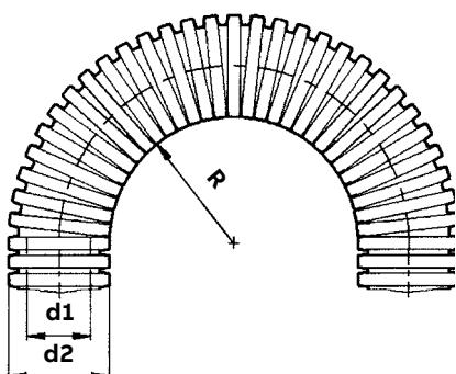
**Stat. radius** = Lowest recommended bending radius for static (fixed) installation.
