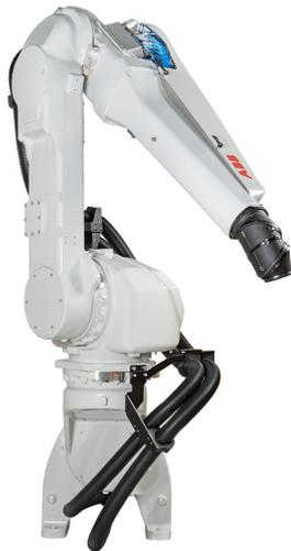
IRB 5500-27 is a new variant of the innovative IRB 5500 robot family. Featuring integrated 7-axes that enable a wider working range and flexible installation positioning, IRB 5500-27 is capable of supporting both interior and exterior automotive painting, as well as other paint applications.
