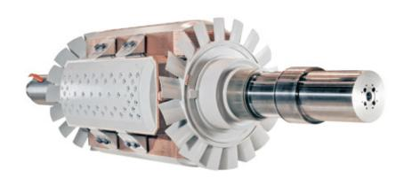
Upgrading a motor's or generator's rotor during a L4-maintenance program is a time and cost efficient opportunity to improve an installation. The latest rotor technology features improved thermal and mechanical strength for higher reliability. Depending on the installation, it can extend rotor design life by some 15 percent and increase power output in excess of 5 percent.
