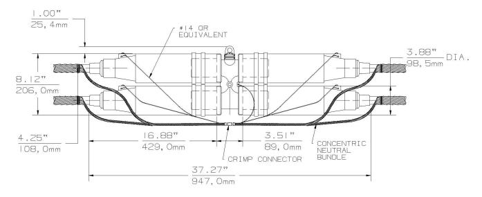
Note. Drawing is a reference only, does not includes cable adapters and lugs, just housing and bus.
