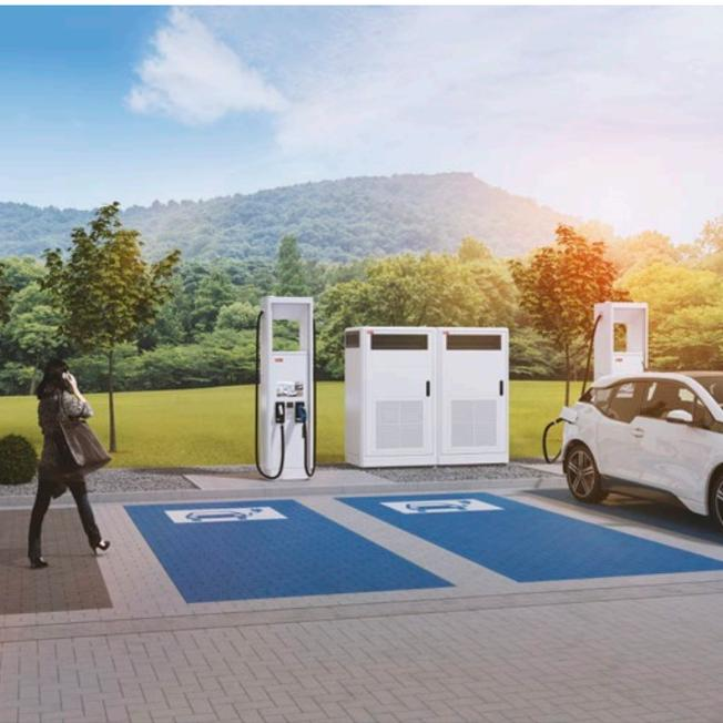
Terra HP is a modular high power charging system with high output current capability, supporting both 400 V<sub>DC</sub> and 800 V<sub>DC</sub> vehicles. A single power cabinet system can deliver up to 375 A and 160 kW continuously, and 175 kW peak. With two power cabinets the system delivers up to 500 A and 350 kW.
