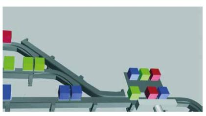
03 ACOPOStrak's purely electromagnetic diverters divide and merge product flows at full production speed.
