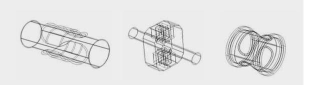
Integration of physical phenomena Initially, the geometry of a flowmeter was constructed using a computer-aided design (CAD) software  $\rightarrow$ 2a. The geometry, or the computational
