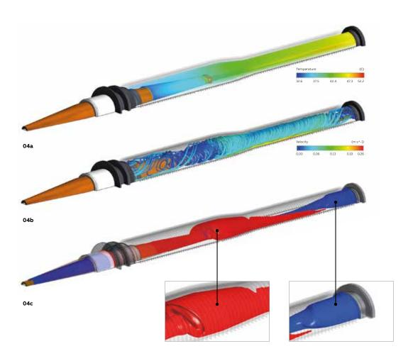
04 Examples of the results given by numerical simulations. 04a Temperature distribution. 04b Velocity streamlines. 04c Temperature isosurfaces.
