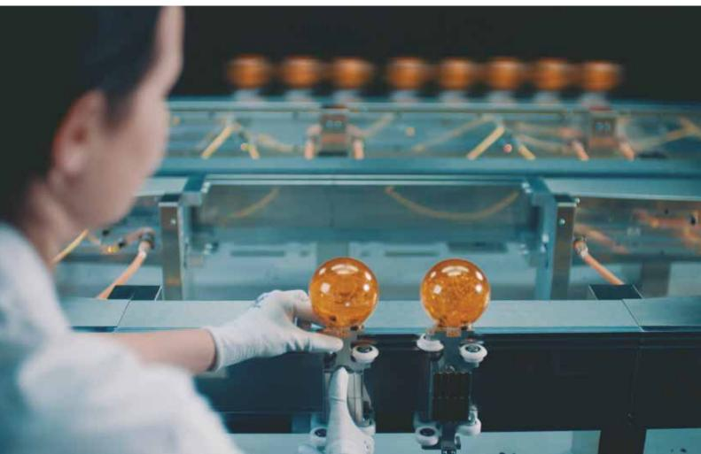
ACOPOStrak's absolute design flexibility allows it to morph into all types of open and closed layouts by arranging the segments in different combinations on a grid  $\rightarrow 6$ . The core of the track system is a linear motor assembled from four types of modular segments: a straight segment, a 45° segment and two 22.5° segments – one curved to the right, the other to the left.
