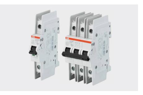
The miniature circuit breaker SU 200 M is ABB's solution for UL 489 branch circuit protection up to 480 Y/277 V AC and 96 V DC. This circuit breaker is an all-round device for AC and DC applications for universal use in North American and global markets due to its approvals acc. to the international standards UL, CSA and IEC. Moreover, SU 200 M is fully compatible with System pro M compact® UL 489 accessories.
