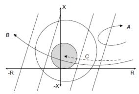
Figure 5: Example of out of step detection
