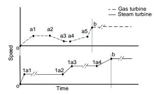
Figure 2, Start up sequence speed vs time
