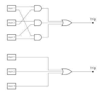
Fig. 1. Protection scheme with three relays in the two-out-of-three voting scheme (above) and redundant scheme with three relays (below). In the first, at least two relays must send a trip signal in order to trigger the trip, while in the latter at least one must be available.
