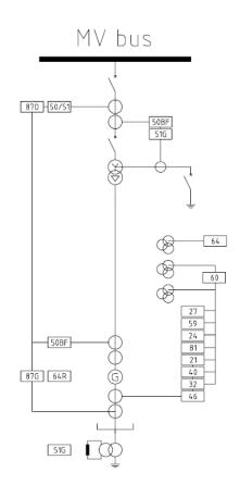
Figure 4, Typical MV Generator Protection Single Line Diagram
