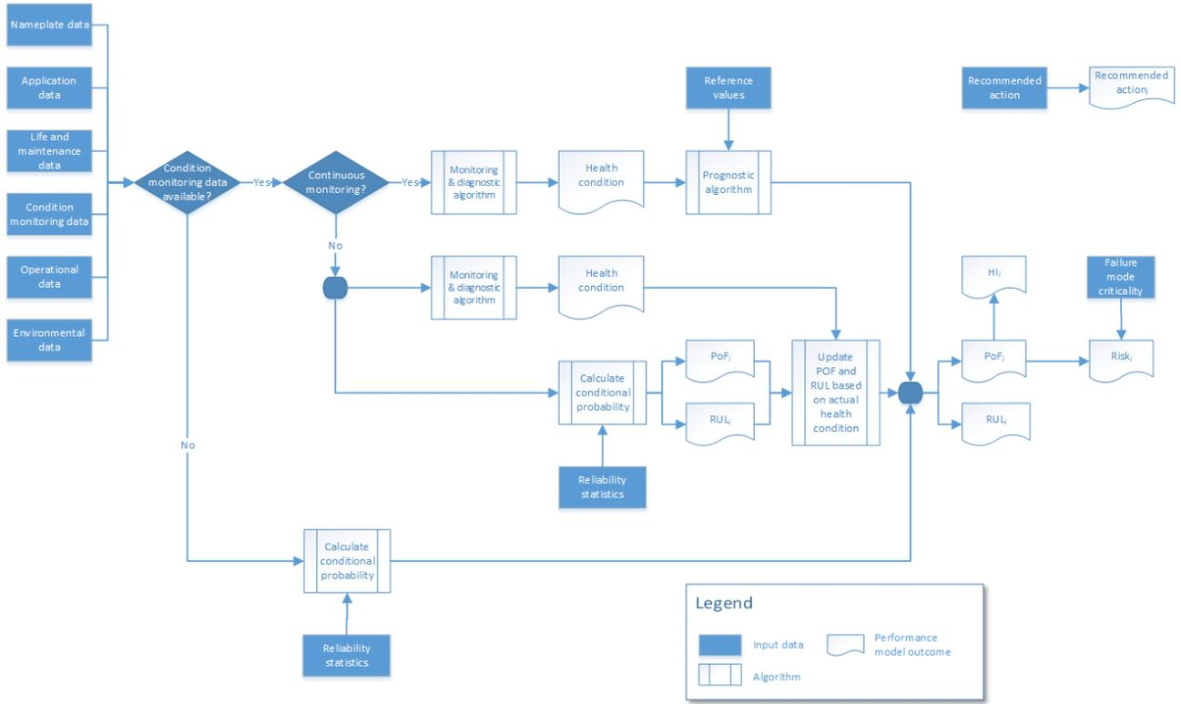
Fig.3 Algorithm for the determination of the outcomes of the performance model for the failure mode  $i$ .
