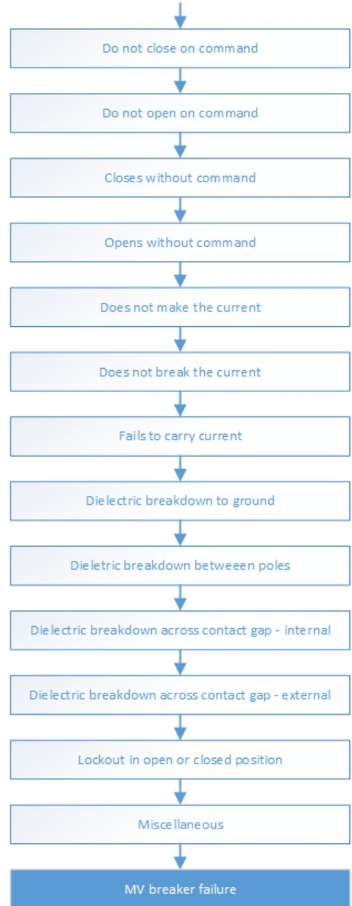
Fig. 2 MV breaker as series of failure modes.
