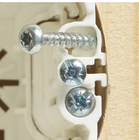
The box can be mounted on, for example, a timber wall or wooden frame with inclined screws (the maximum size of fastening screw head Ø 6 mm).
