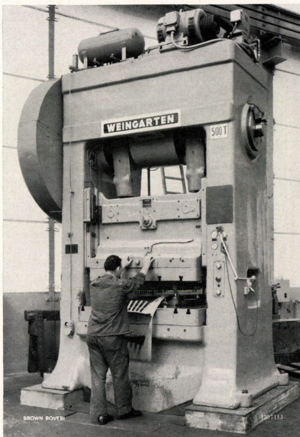
Fig. 2. - Pressing single magnet segments, two-hand release
