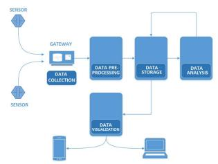
Figure 2 Information flow in the ABB Ability  $^{\rm TM}$
