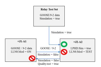
Figure 5. Periodical testing connecting relay test set to IEC 61850 communication bus
