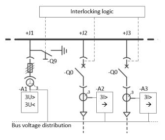
Figure 3. Reference application with bus voltage sharing and interlocking using hard-wired signals.
