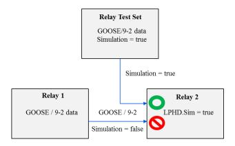
Figure 2. Simulation according IEC 61850
